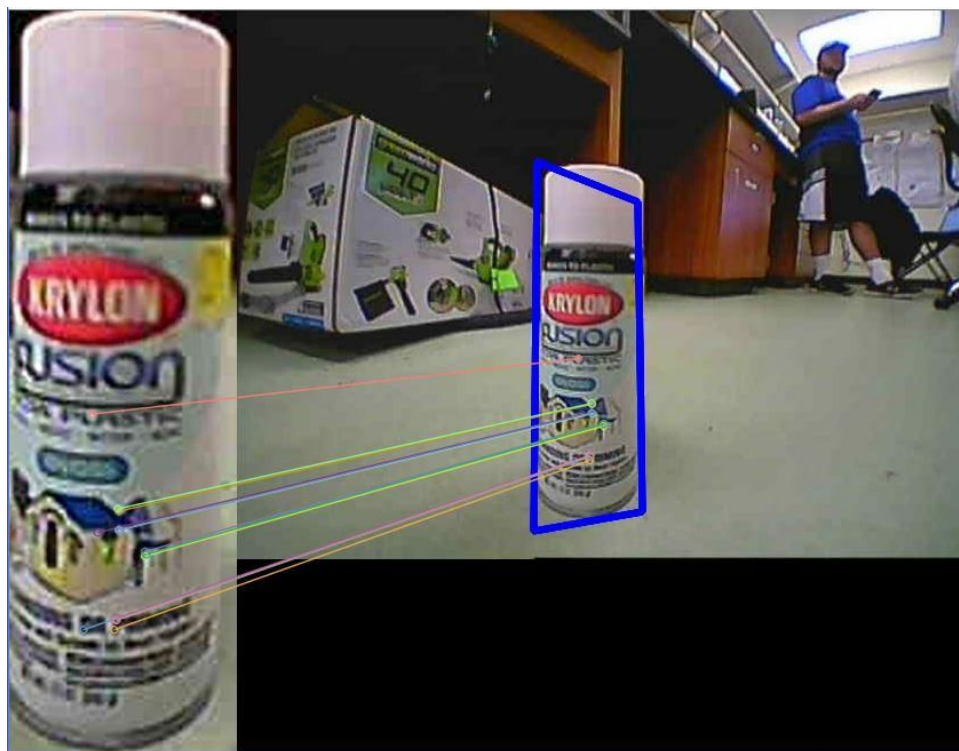
Figure III – Feature Matching Prototype System
